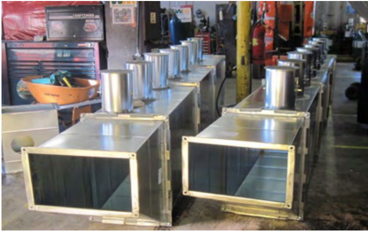
Duct, pictured above, is fabricated with small take-offs, dampers and bird screen to exhaust evenly from each trapped ceiling pocket cavity.
